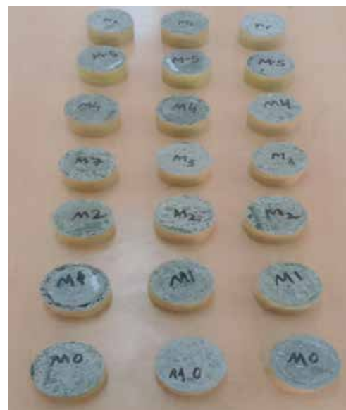
Fig. 5 Test samples before and during RCPT Tests
