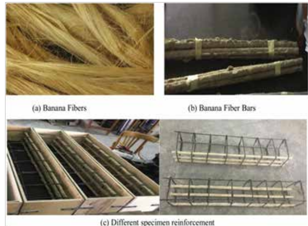
Figure 2: Details of specimen for reinforcement
