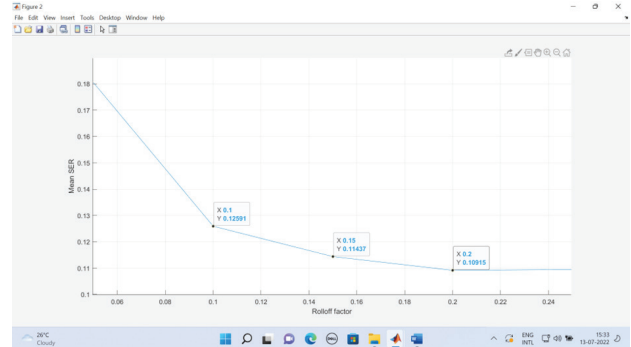
Graph 4: Output result Mean SER between roll-off factor with carrier frequency offset in GFDm
